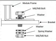
Fig. 7 Diagram of the bolt installation process
