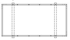
Fig 4. Outer four-hole bolt installation for 72cell
