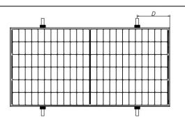
Fig. 8 Rails vertical to the long-side frame
