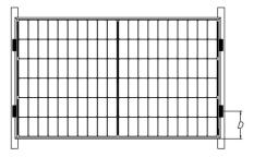
Fig. 9 Rails overlapping the short-side frame
