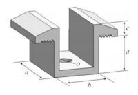
Fig. 10 Schematic diagram of the mid clamp
