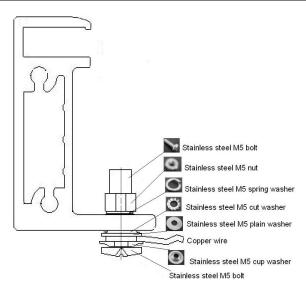
Fig. 15 Grounding the aluminum frame with copper wire
